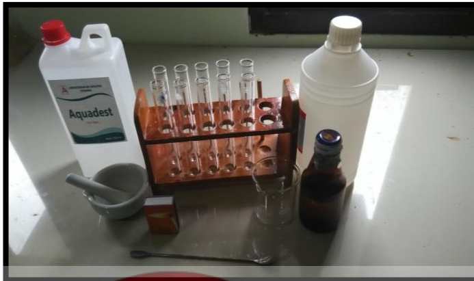
Gambar 1. Tabung Reaksi, Rak Tabung, Larutan H_2SO_4 Peekat, Aquadest, Methanol 95%, Cawan Porselen, Batang Pengaduk, Korek Api, Beker Glass
