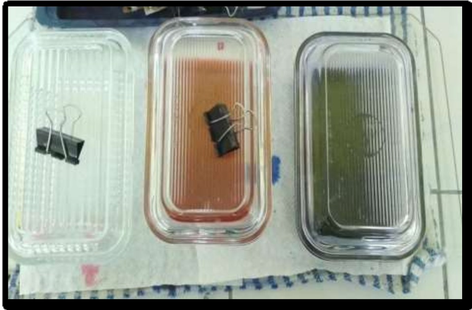
Gambar 1. Reagen Rapid Staining , Reagensia 1 Methanol (Larutan Fiksas), Reagensia 2 (Larutan Eosin ), Reagen 3 (Larutan Methylen Blue )
