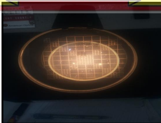
Gambar 6. Perhitungan bakteri di alat colony counter
